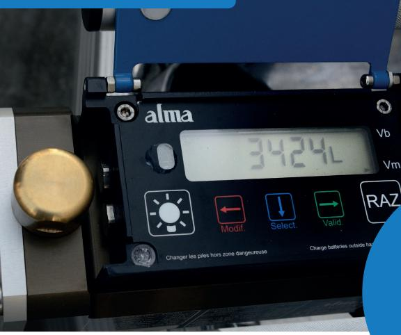
approved, portable gravity flow meter for petroleum products
